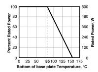
Derating (thermal resistance): 8.33 W/K (0.12 K/W) (for conf. 1, 2, 3) Best results can be obtained by using a thermal transfer compound with a heat conductivity of at least 2.9 W/mK. The flatness of the cooling plate must be better than 0.05 mm overall. Surface roughness should not exceed 6.4  $\mu$ m.
