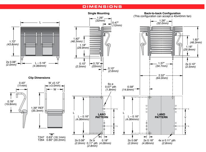
NOTE: Due to possible screw torquing on long extrusions, Customer should check for coplanarity prior to final assembly or soldering.
