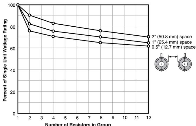
Fig. 6: Derating of Resistors to Allow for Grouping
